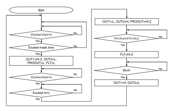
Figure 12. SCP Operation Status Transition Diagram
