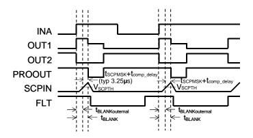
Figure 10. DESAT Operation Timing Chart
