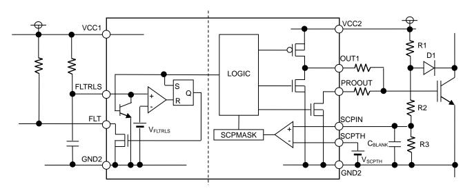
Figure 9. Block Diagram for DESAT
