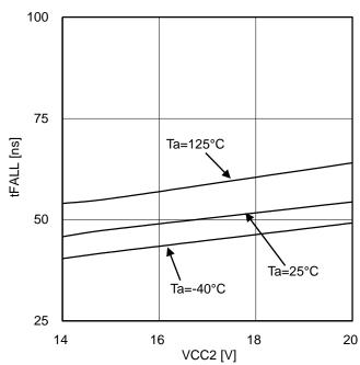
Figure 41. Fall time (10000pF between OUT1-GND2)
