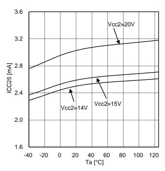
Figure 25. Output side circuit current (at OUT1=L)
