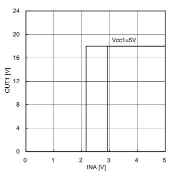
Figure 29. Logic (INA/INB) High/Low level input voltage at Ta=25°C
