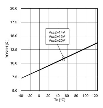
Figure 42. OUT2 ON resistance (Source)
