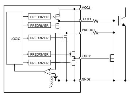
Figure 3. Block diagram of Miller Clamp function
