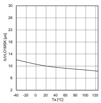
Figure 47. VCC1 UVLO mask time
