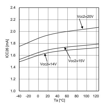
Figure 27. Output side circuit current (at OUT1=H)
