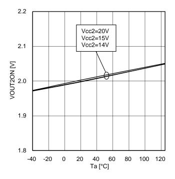
Figure 44. OUT2 ON threshold voltage
