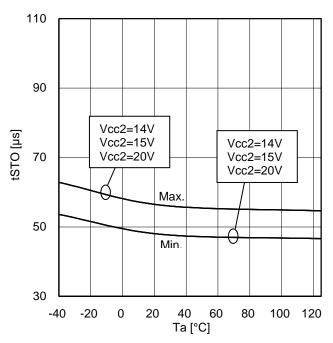
Figure 52. Soft turn OFF release time
