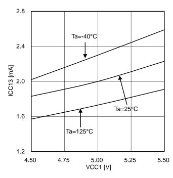
Figure 20. Input side circuit current (at INA=10kHz and Duty=50%)
