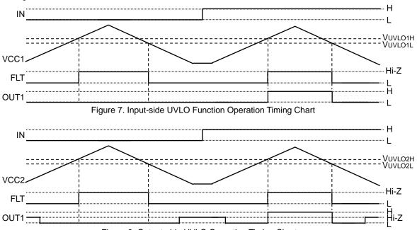
Figure 8. Output-side UVLO Operation Timing Chart
