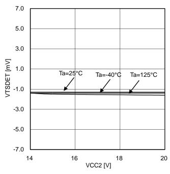
Figure 53. VTS offset voltage (at VTSTH=1.7V)
