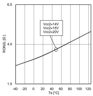
Figure 43. OUT2 ON resistance (Sink)
