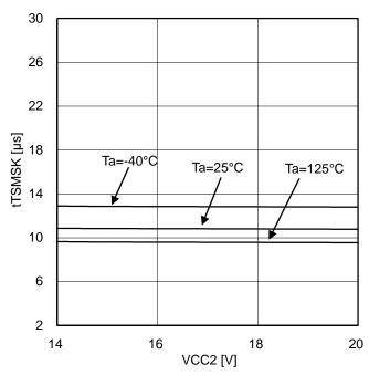
Figure 54. Thermal detection mask time
