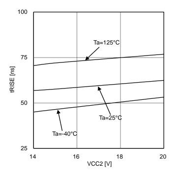
Figure 40. Rise time (10000pF between OUT1-GND2)
