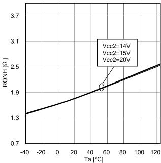
Figure 35. OUT1 ON resistance (Source)
