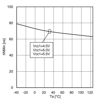
Figure 31. Logic input minimum pulse width (H pulse)
