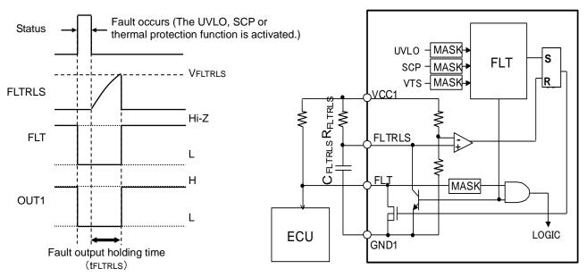
Figure 5. Fault Status Output Timing Chart
