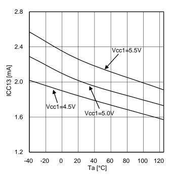
Figure 21. Input side circuit current (at INA=10kHz and Duty=50%)
