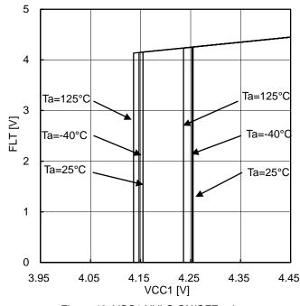
Figure 46. VCC1 UVLO ON/OFF voltage
