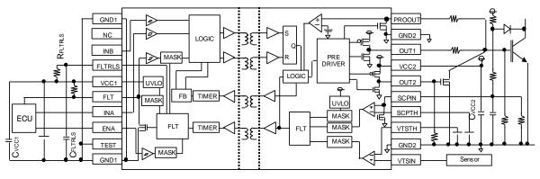
Figure 2. For using 3-pin IGBT (for using DESAT function)
