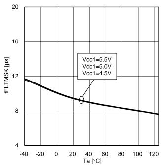
Figure 32. Logic input minimum pulse width (L pulse)
