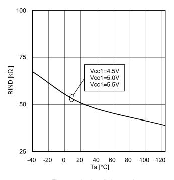
Figure 30. Logic pull-down resistance
