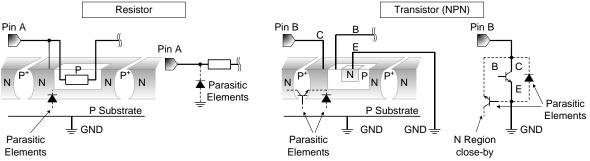
Figure 60. Example of monolithic IC structure
