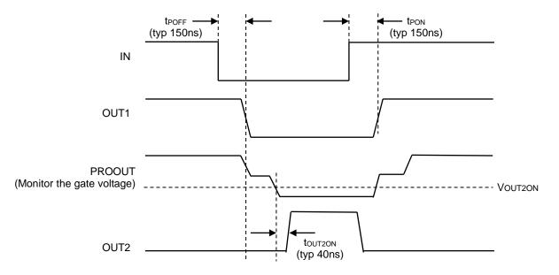
Figure 4. Timing chart of Miller Clamp function
