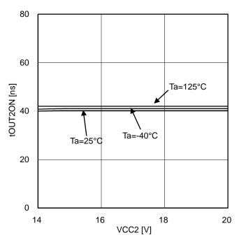
Figure 45. OUT2 output delay time
