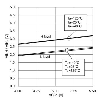
Figure 28. Logic (INA/INB) High/Low level input voltage
