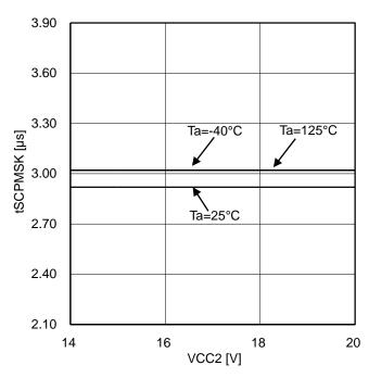
Figure 51. SCP detection mask time
