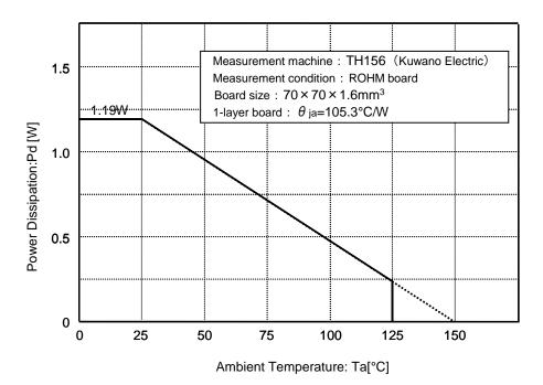
Figure 59. SSOP-B20W Derating Curve
