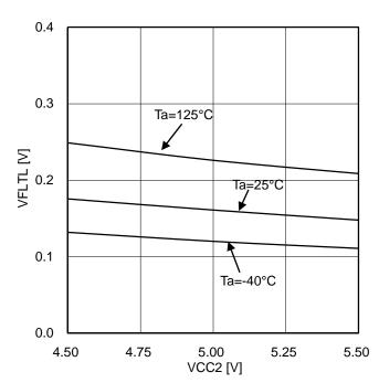
Figure 55. FLT output low voltage (IFLT=5mA)
