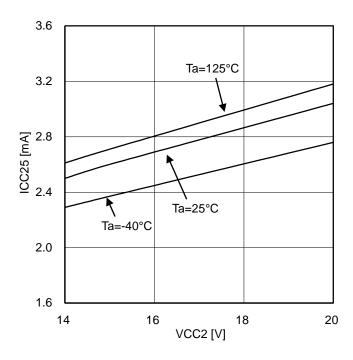
Figure 24. Output side circuit current (at OUT1=L)
