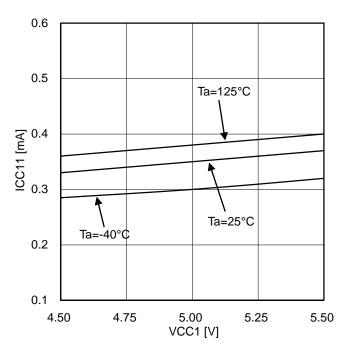
Figure 16. Input side circuit current (at OUT1=L)
