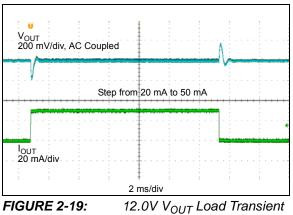
FIGURE 2-19: Waveforms.
