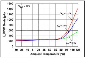
**FIGURE 2-10:** No Load Input Current, I<sub>INO</sub> vs. Ambient Temperature.
