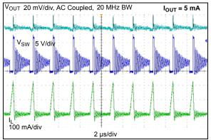
**FIGURE 2-15:** 12.0V VOUT Light Load PWM Mode Waveforms.
