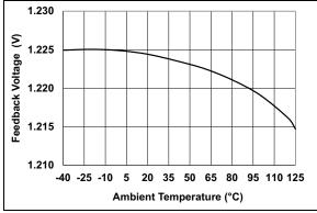
FIGURE 2-2: V<sub>FB</sub> Voltage vs. Ambient Temperature and V<sub>IN.</sub>
