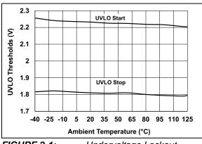
FIGURE 2-1: Undervoltage Lockout (UVLO) vs. Ambient Temperature.
