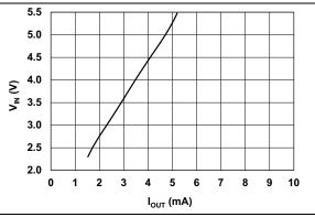
FIGURE 2-12: PWM Pulse Skipping Mode Threshold.
