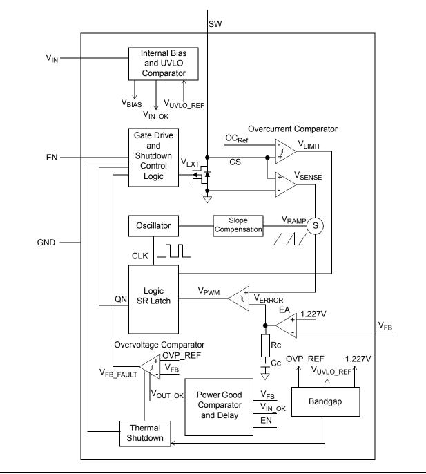
FIGURE 4-1: MCP1663 Simplified Block Diagram.
