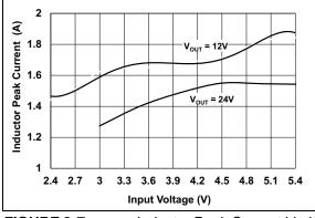
FIGURE 2-7: Inductor Peak Current Limit vs. Input Voltage.
