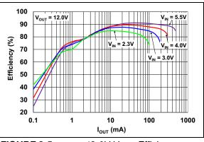
**FIGURE 2-5:** 12.0V V<sub>OUT</sub> Efficiency vs. I<sub>OUT</sub>.
