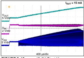
**FIGURE 2-18:** 12.0V Start-Up  $(V_{IN} = V_{ENABLE}).$
