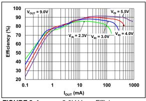
**FIGURE 2-4:** 9.0V V<sub>OUT</sub> Efficiency vs. I<sub>OUT</sub>.
