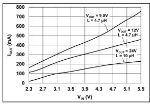
FIGURE 2-3:Maximum Output Currentvs.  $V_{IN}$  ( $V_{OUT}$  in Regulation with Max. 5% Drop).
