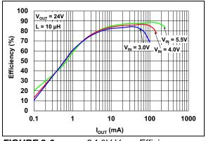
**FIGURE 2-6:** 24.0V V<sub>OUT</sub> Efficiency vs. I<sub>OUT</sub>.
