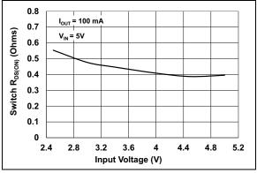
FIGURE 2-14: N-Channel Switch R<sub>DSON</sub> vs. V<sub>IN</sub>.
