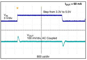
12.0V V<sub>OUT</sub> Line Transient FIGURE 2-20: Waveforms.
