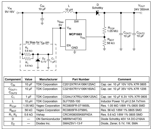
**FIGURE 6-6:** High Voltage (9 to 16V) Input Boost Converter to 24V Output with Separate 5V Bias for V<sub>IN</sub> pin.
