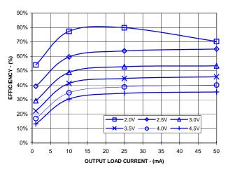
Figure 14 – Efficiency vs. Output Current;  $T_A = 25^{\circ}C$ ,  $C1 = 0.22\mu F$ , C2, C3,  $C4 = 4.7\mu F$ ,  $C_{FILT} = 0.1\mu F$
