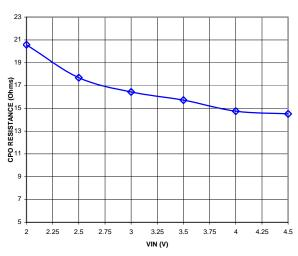
Figure 7 – CPO Output Resistance vs. Input Voltage;  $T_A = 25^{\circ}C,~C1 = 0.22\mu F,~C2,~C3,~C4 = 4.7\mu F,~C_{FILT} = 0.1\mu F$
