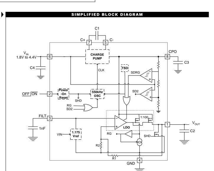
Figure 2 – LX1882-33 Block Diagram
