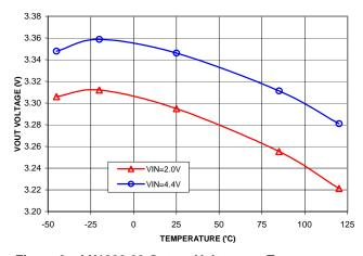
Figure 9 – LX1882-33 Output Voltage vs. Temperature; C1 = 0.22 $\mu$ F, C2, C3, C4 = 4.7 $\mu$ F, C<sub>FILT</sub> = 0.1 $\mu$ F
