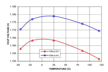
Figure 10 – LX1882-00 Output Voltage vs. Temperature;  $C1 = 0.22\mu F, C2, C3, C4 = 4.7\mu F$
