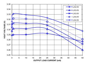
Figure 8 – LX1882-33 Output Voltage vs. Load Current;  $T_A = 25^{\circ}C,~C1 = 0.22\mu F,~C2,~C3,~C4 = 4.7\mu F,~C_{FILT} = 0.1\mu F$
