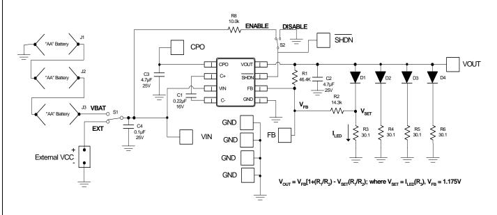
Figure 6 – LX1882-00 Evaluation Board Schematic; LED Driver Application
