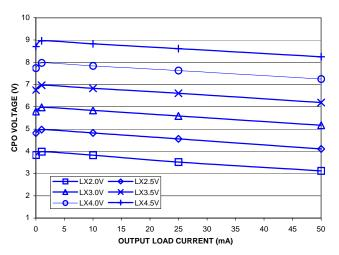
Figure 11 – CPO Voltage vs. Input Voltage;  $T_A = 25^{\circ}C$ ,  $C1 = 0.22\mu F$ , C2, C3,  $C4 = 4.7\mu F$ ,  $C_{FILT} = 0.1\mu F$
