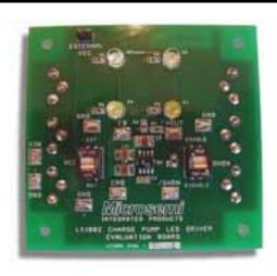
Figure 4. LX1882 LED Driver Evaluation Board (Top View)
