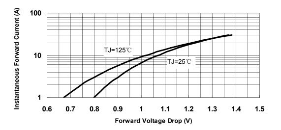
Fig.3-Typical Instantaneous Forward Voltage Characteristics
