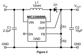
Boost regulation is achieved by turning on an internal switch, which draws current through the inductor (L1). When the switch turns off, the inductor's magnetic field collapses, causing the current to be discharged into the output capacitor through an external Schottkey diode (D1). Voltage regulation is achieved my modulating the pulse width or pulse width modulation (PWM).
