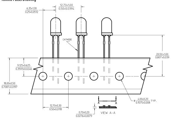
$Note: The\ ammo-packs\ drawing\ is\ applicable\ for\ packaging\ option\ -DD\ \&\ -ZZ\ and\ regardless\ standoff\ or\ non-standoff\ or\ no$
