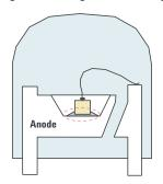
Note: Electrical connection between bottom surface of LED die and the lead frame is achieved through conductive paste.
