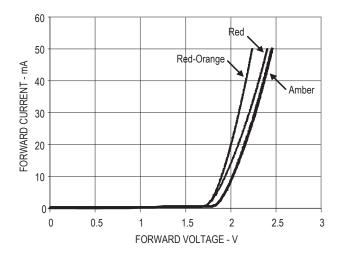
Figure 2. Forward current vs. forward voltage
