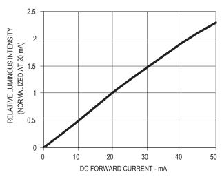
Figure 3. Relative luminous intensity vs. forward current
