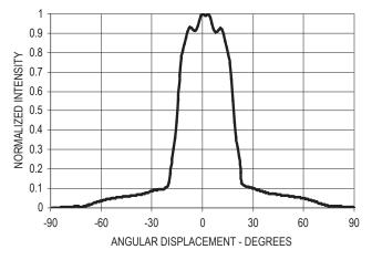
Figure 7. Representative spatial radiation pattern for  $30^\circ$  viewing angle lamps
