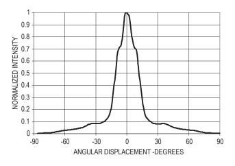
Figure 6. Representative spatial radiation pattern for 23  $^{\circ}$  viewing angle lamps
