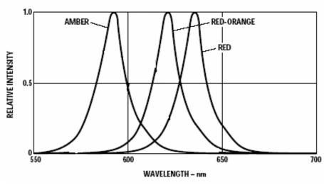
Figure 1. Relative intensity vs. peak wavelength
