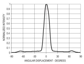
Figure 5. Representative spatial radiation pattern for 15  $\!\!^\circ$  viewing angle lamps
