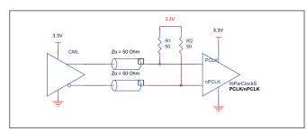
FIGURE 4A. PCLK/NPCLK INPUT DRIVEN BY A CML DRIVER
