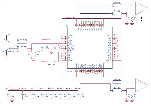
FIGURE 5. 8524 HSTL BUFFER SCHEMATIC EXAMPLE
