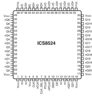
64-Lead TQFP E-Pad 10mm x 10mm x 1.0mm package body Y package Top View
