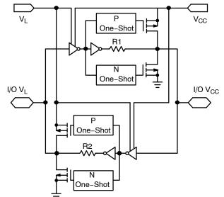
Figure 2. Simplified Functional Diagram (1 I/O Line)
