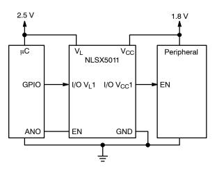
Figure 4. Application Example for  $V_L > V_{CC}$
