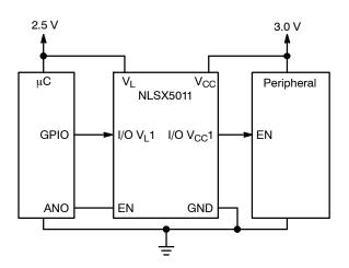
Figure 3. Application Example for V<sub>L</sub> < V<sub>CC</sub>
