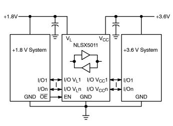
Figure 1. Typical Application Circuit
