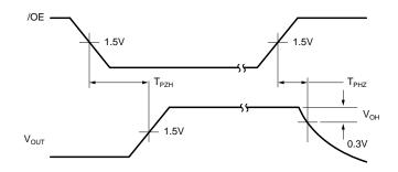
Figure 2. 3-State Output High Enable and Disable Times
