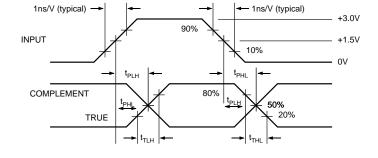
Figure 4. Propagation Delay and Transition Times
