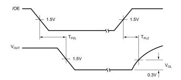
Figure 1. 3-State Output Low Enable and Disable Times
