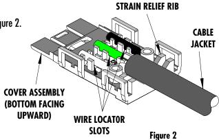
3. Position wires into locator slots. Be certain to place black wire in slot marked BLK, green wire in slot marked GRD, and the white wire in the third slot. Upon final positioning of all wires, be certain the end of the cable jacket is a minimum of .06" past the second strain relief rib as shown in Figure 2.
